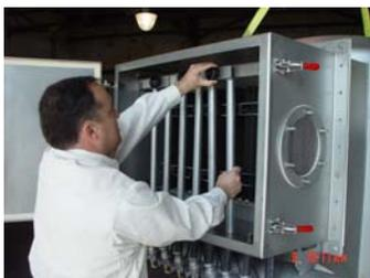
(J) Replacing and tightening hold-down knobs
