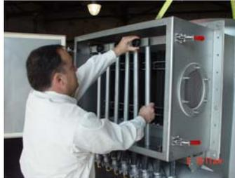
(B) Loosening and removing hold-down knobs
