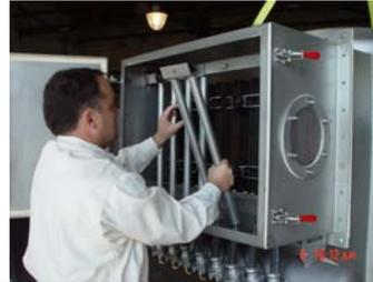
(C) Removing air distribution tubes.
