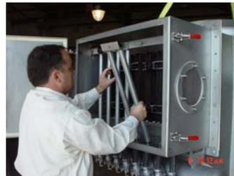
(I) Installing air distribution tubes
