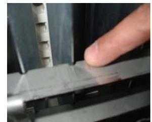
(O) Retainers are notched for proper venturi alignment
