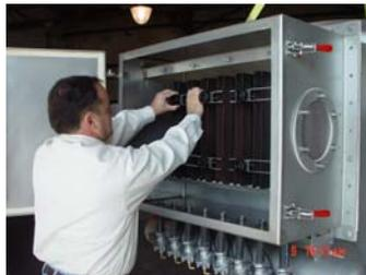
(H) Installing venturies and retainers
